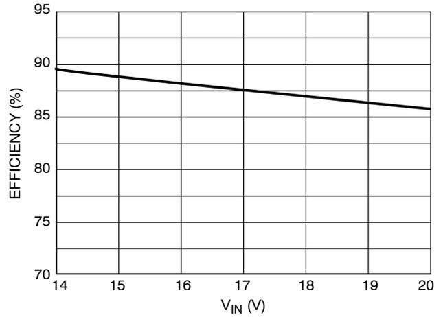
**Figure 15. 12 V<sub>AC</sub> Input 5 W LED Driver Efficiency**
