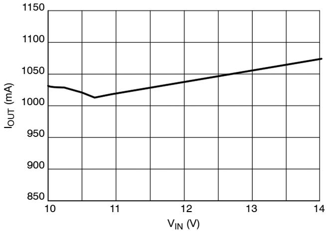
**Figure 14. Current Regulation, 12 V<sub>DC</sub> Input 5 W LED Driver**
