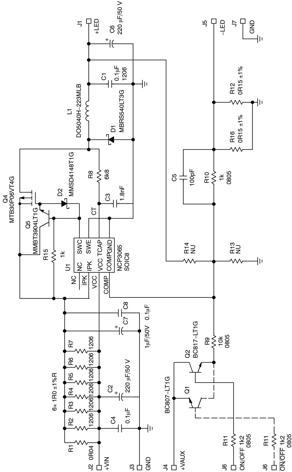
Figure 9. NCP3065 3A Buck Evaluation Board Schematic
