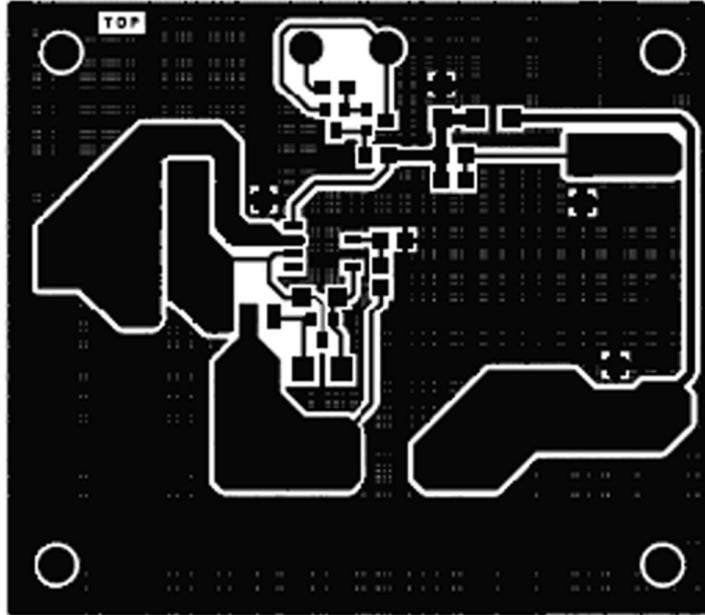
Figure 7. Evaluation Board Layout Top (Not in Scale)
