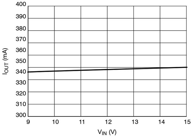
**Figure 12. Current Regulation, 12 V<sub>DC</sub> Input 1 W LED Driver**
