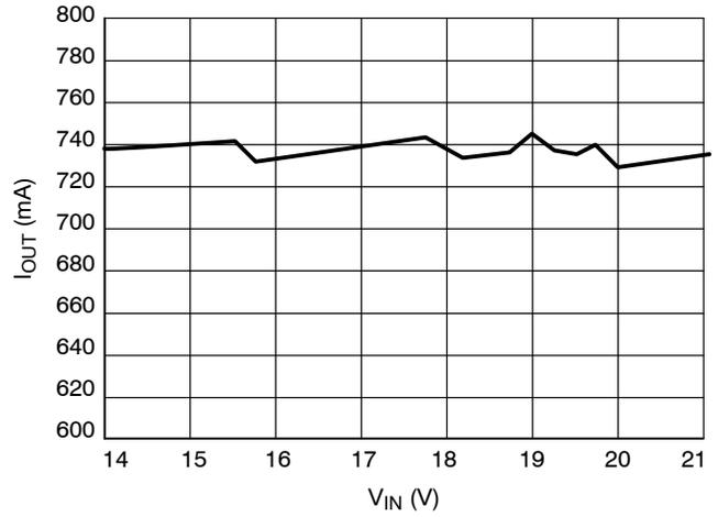
**Figure 13. Current Regulation, 12 V<sub>AC</sub> Input 3 W LED Driver**
