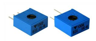
The Model 63 cermet trimmer is available in several pin configurations for top or side adjustment and with a choice of Knob styles for finger setting. Quick adjustment is achieved with multi-finger wiper and the standard resistance range is between 100  $\Omega$  and 2 M $\Omega$  with a tolerance of  $\pm$  10 %.
