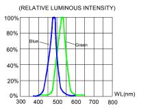
FIG.4 RELATIVE LUMINOUS INTENSITY VS. WAVELENGTH.
