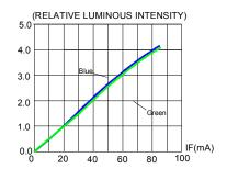
FIG.2 RELATIVE LUMINOUS INTENSITY VS. FORWARD CURRENT
