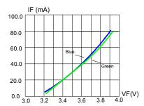
FIG.1 FORWARD CURRENT VS. FORWARD VOLTAGE.
