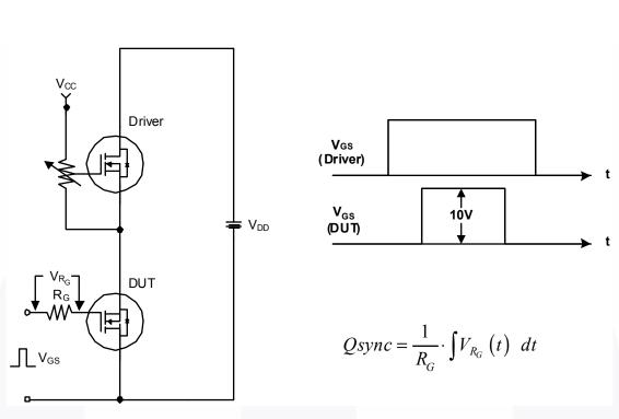
Figure 18. Total Gate Charge Qsync. Test Circuit & Waveforms
