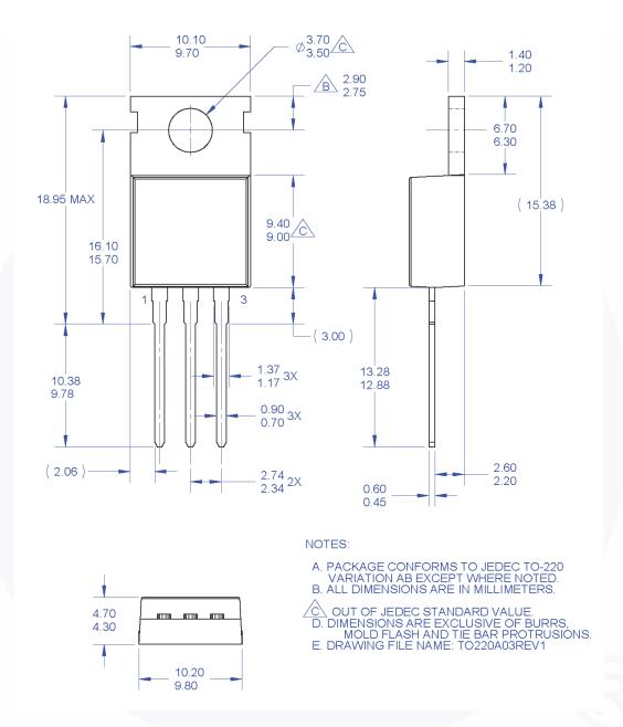
Figure 19. TO220, Molded, 3-Lead, Jedec Variation AB, Non Jedec F102
