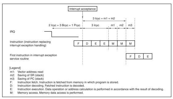
Figure 6.4 Example of Pipeline Operation when IRQ Interrupt is Accepted (No Register Banking)
