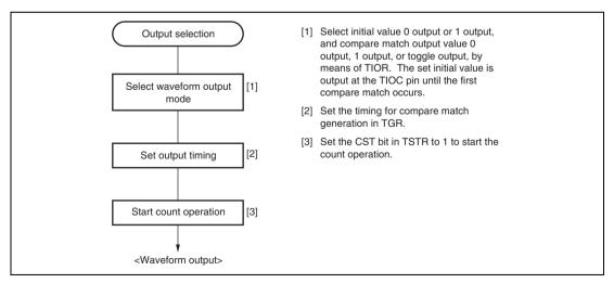
Figure 10.7 Example of Setting Procedure for Waveform Output by Compare Match
