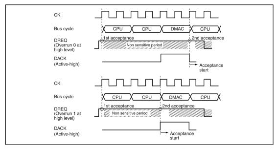
Figure 9.14 Example of DREQ Input Detection in Cycle Steal Mode Level Detection
