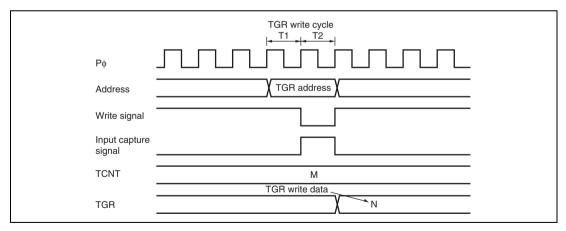
Figure 10.127 Contention between TGR Write and Input Capture (Channel 5)
