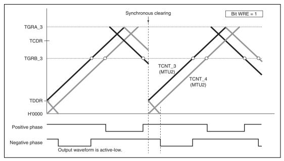
Figure 10.60 Example of Synchronous Clearing in Dead Time during Down-Counting (Timing (8) in Figure 10.56; Bit WRE of TWCR is 1)
