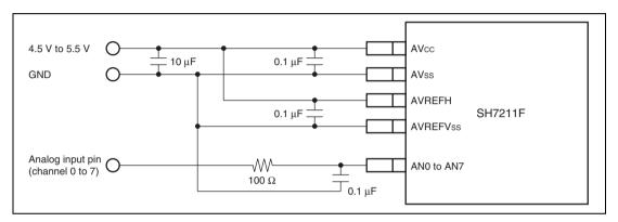
Figure 17.8 Example of Analog Input Pin Protection Circuit
