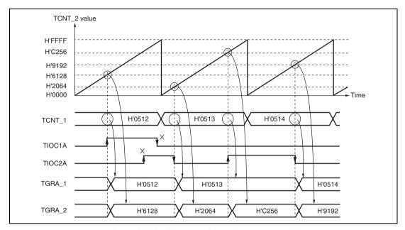
Figure 10.23 Cascaded Operation Example (c)
