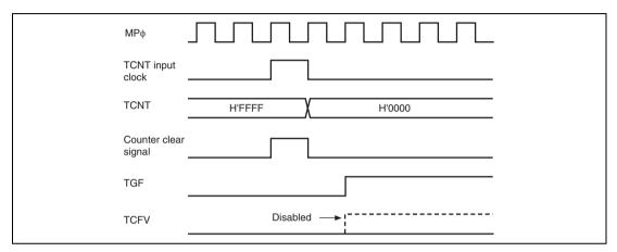
Figure 10.133 Contention between Overflow and Counter Clearing
