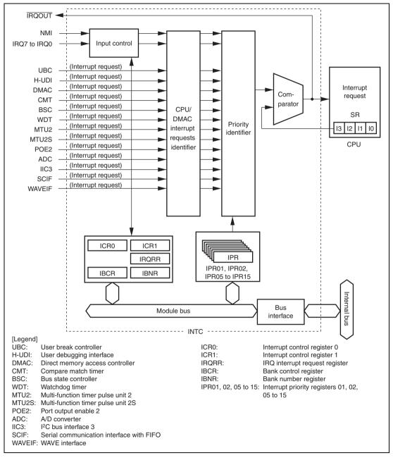
Figure 6.1 Block Diagram of INTC
