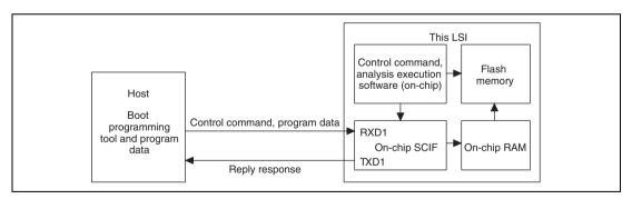
Figure 21.6 System Configuration in Boot Mode
