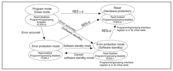
Figure 21.16 Transitions to and from Error Protection State
