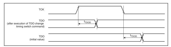
Figure 24.3 H-UDI Data Transfer Timing
