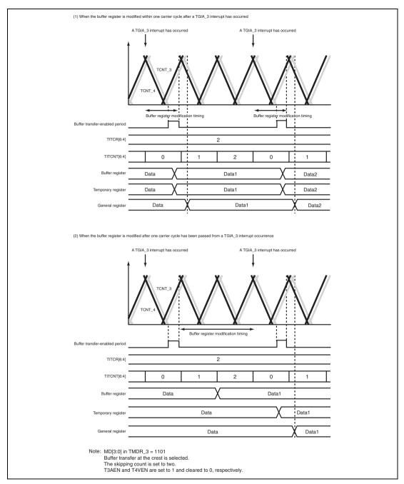
Figure 10.77 Example of Operation when Buffer Transfer is Linked with Interrupt Skipping (BTE1 = 1 and BTE0 = 0)
