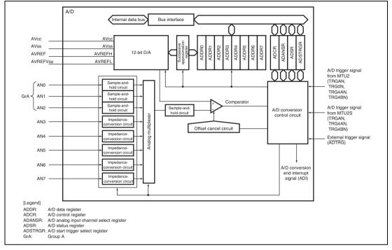
Figure 17.1 Block Diagram of A/D Converter
