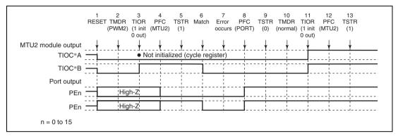
Figure 10.147 Error Occurrence in PWM Mode 2, Recovery in Normal Mode
