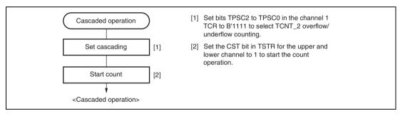
Figure 10.20 Cascaded Operation Setting Procedure
