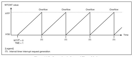
Figure 14.5 Operation in Interval Timer Mode
