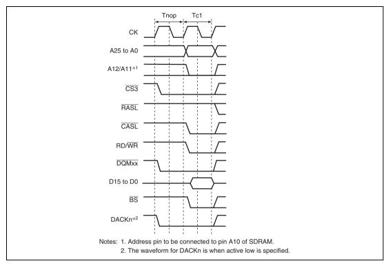
Figure 8.23 Single Write Timing (Bank Active, Same Row Addresses in the Same Bank)
