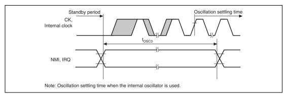
Figure 27.7 Oscillation Settling Time on Return from Standby (Return by NMI or IRQ)
