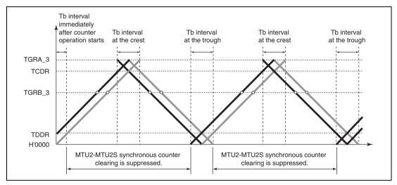
Figure 10.62 MTU2–MTU2S Synchronous Clearing-Suppressed Interval Specified by SCC Bit in TWCR
