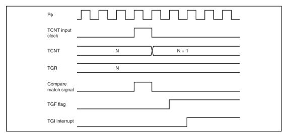
Figure 10.109 TGI Interrupt Timing (Compare Match)
