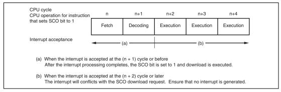
Figure 21.18 Timing of Contention between SCO Download Request and Interrupt Request
