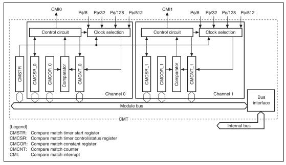
Figure 13.1 Block Diagram of CMT
