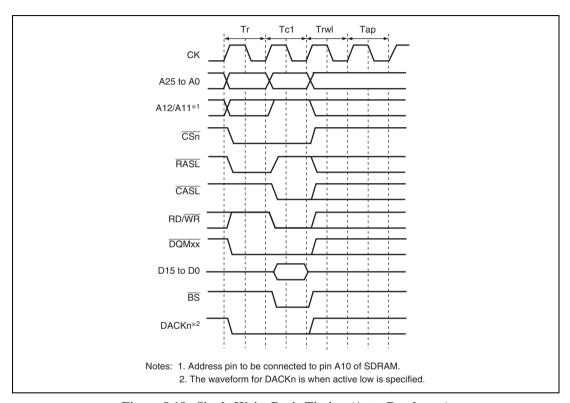
Figure 8.18 Single Write Basic Timing (Auto-Precharge)
