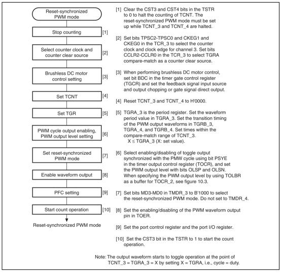
Figure 10.35 Procedure for Selecting Reset-Synchronized PWM Mode
