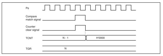
Figure 10.101 Counter Clear Timing (Compare Match) (Channel 5)
