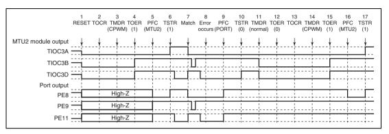
Figure 10.158 Error Occurrence in Complementary PWM Mode, Recovery in Complementary PWM Mode
