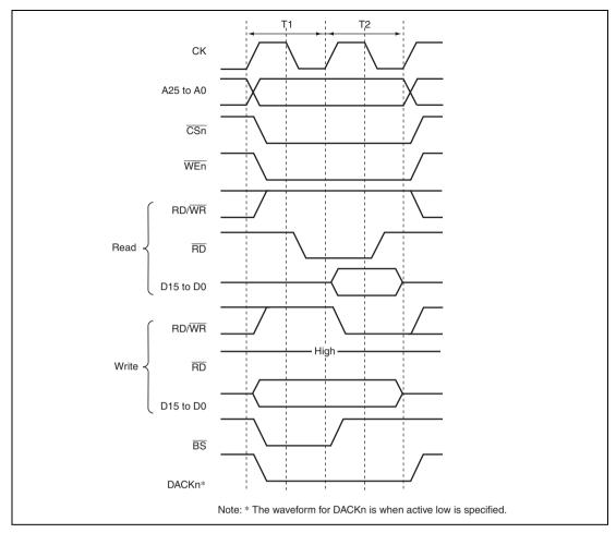
Figure 8.34 Basic Access Timing for SRAM with Byte Selection (BAS = 1)
