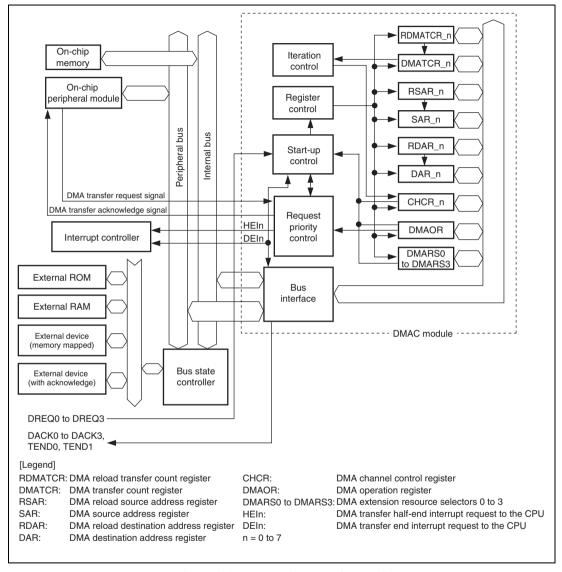
Figure 9.1 Block Diagram of DMAC
