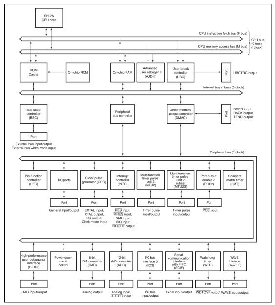
Figure 1.1 Block Diagram
