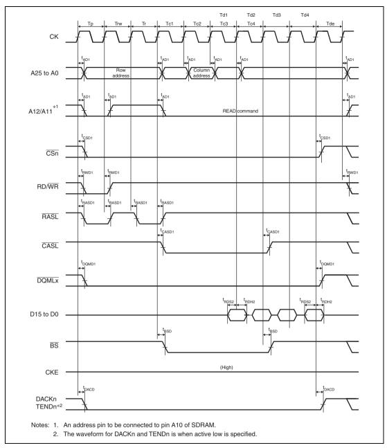
Figure 27.30 Synchronous DRAM Burst Read Bus Cycle (Four Read Cycles)
