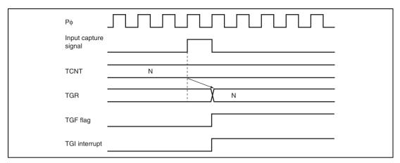
Figure 10.112 TGI Interrupt Timing (Input Capture) (Channel 5)
