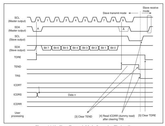
Figure 16.10 Slave Transmit Mode Operation Timing (2)
