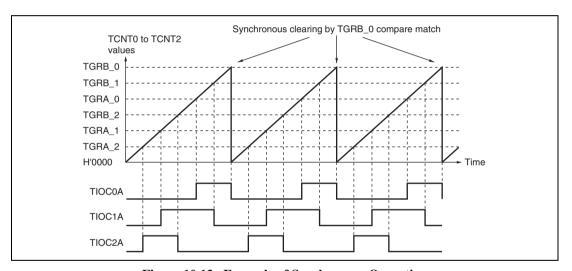
Figure 10.13 Example of Synchronous Operation
