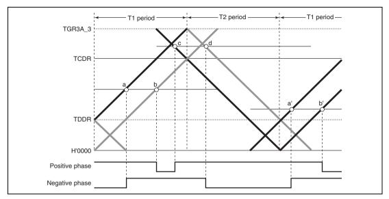
Figure 10.46 Example of Complementary PWM Mode Waveform Output (1)
