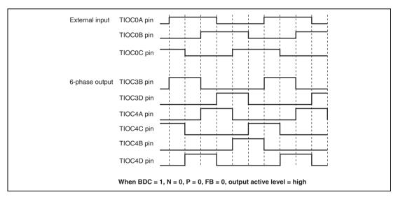
Figure 10.69 Example of Output Phase Switching by External Input (1)
