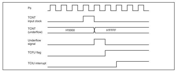
Figure 10.114 TCIU Interrupt Setting Timing
