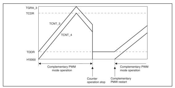
Figure 10.130 Counter Value during Complementary PWM Mode Stop
