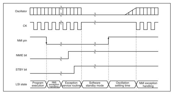
Figure 23.1 NMI Timing in Software Standby Mode (Application Example)
