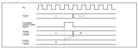
**Figure 10.103 Buffer Operation Timing (Compare Match)**
