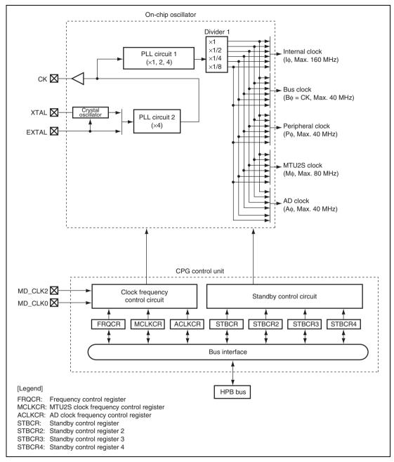
Figure 4.1 Block Diagram of Clock Pulse Generator
