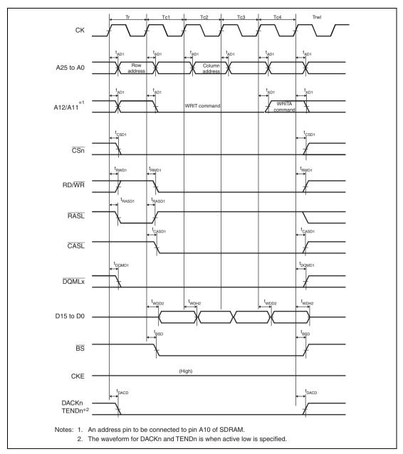
Figure 27.26 Synchronous DRAM Burst Write Bus Cycle (Four Write Cycles)
