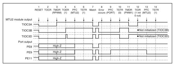
Figure 10.161 Error Occurrence in Reset-Synchronized PWM Mode, Recovery in PWM Mode 1
