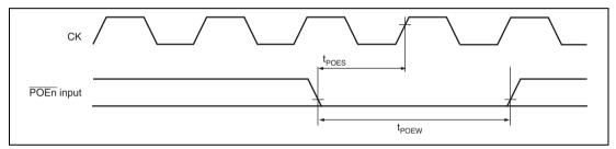
Figure 27.44 POE2 Input/Output Timing
