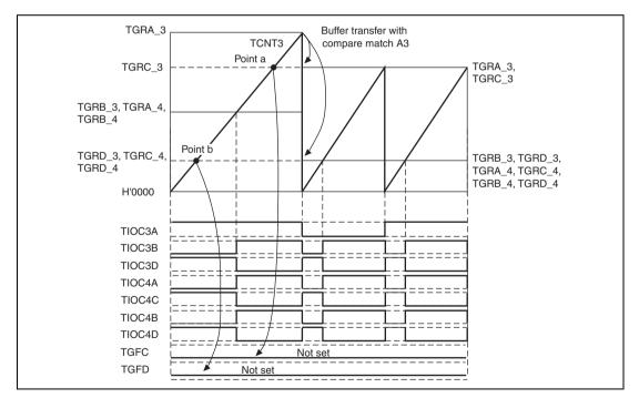
Figure 10.131 Buffer Operation and Compare-Match Flags in Reset Synchronous PWM Mode
