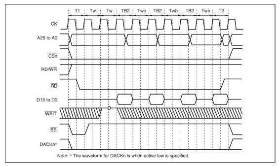
Figure 8.32 Burst ROM Access Timing (Clock Asynchronous)
