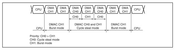
Figure 9.12 Bus State when Multiple Channels are Operating
