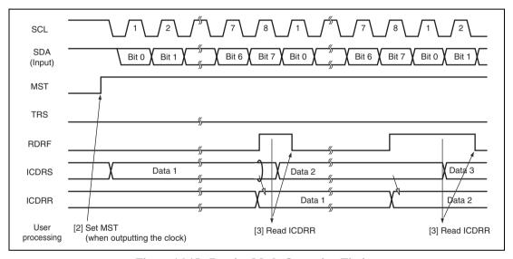
Figure 16.15 Receive Mode Operation Timing
