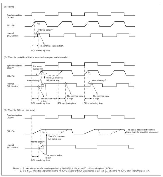
Figure 16.22 Bit Synchronous Circuit Timing
