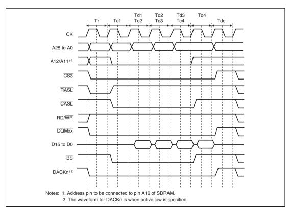
Figure 8.19 Burst Read Timing (Bank Active, Different Bank, CAS Latency 1)
