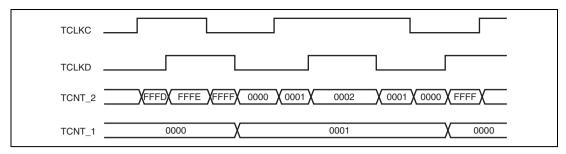
Figure 10.21 Cascaded Operation Example (a)
