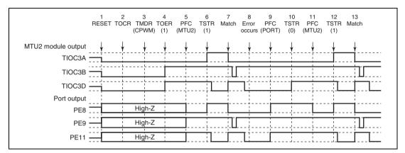
Figure 10.157 Error Occurrence in Complementary PWM Mode, Recovery in Complementary PWM Mode
