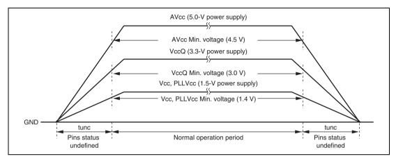
Figure 27.1 Power-on/Power-off Sequence
