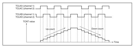
Figure 10.30 Example of Phase Counting Mode 1 Operation
