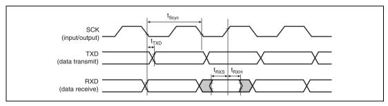
Figure 27.47 SCIF Input/Output Timing in Clocked Synchronous Mode
