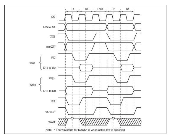
Figure 8.3 Continuous Access for Normal Space 1
