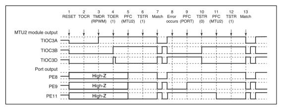
Figure 10.163 Error Occurrence in Reset-Synchronized PWM Mode, Recovery in Reset-Synchronized PWM Mode
