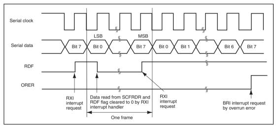
Figure 15.15 Example of SCIF Receive Operation
