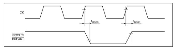
Figure 27.11 Bus Release Timing
