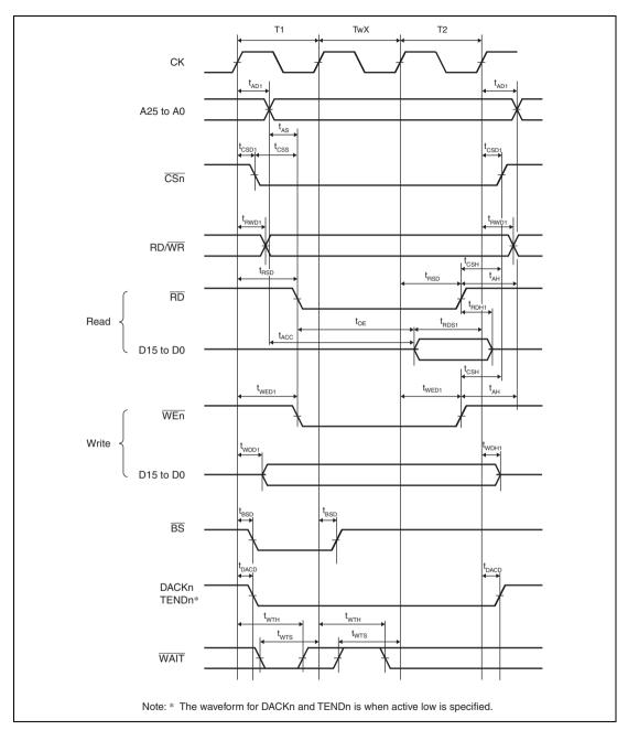
Figure 27.14 Basic Bus Timing for Normal Space (One External Wait Cycle)
