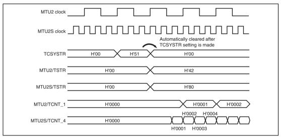
Figure 10.84 (3) Example of Synchronous Counter Start Operation (MTU2-to-MTU2S Clock Frequency Ratio = 1:3)
