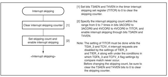
Figure 10.73 Example of Interrupt Skipping Operation Setting Procedure
