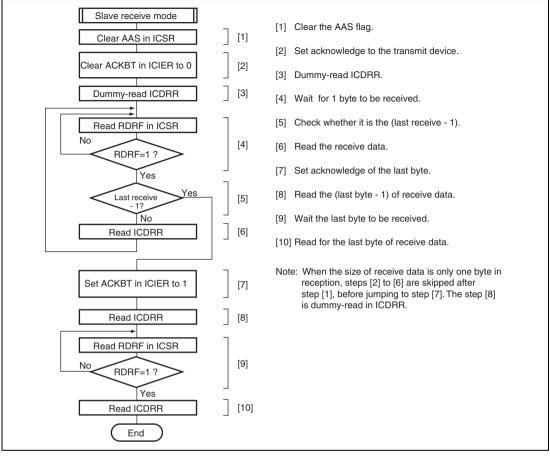
Figure 16.21 Sample Flowchart for Slave Receive Mode
