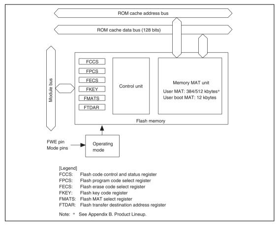
Figure 21.1 Block Diagram of Flash Memory
