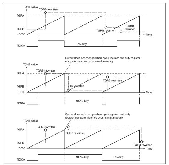
Figure 10.28 Example of PWM Mode Operation (3)
