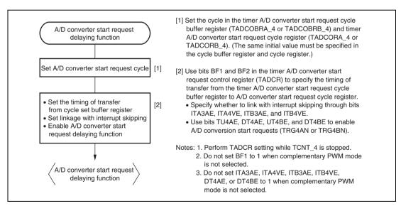
Figure 10.79 Example of Procedure for Specifying A/D Converter Start Request Delaying Function
