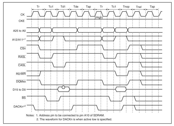
Figure 8.27 Low-Frequency Mode Access Timing
