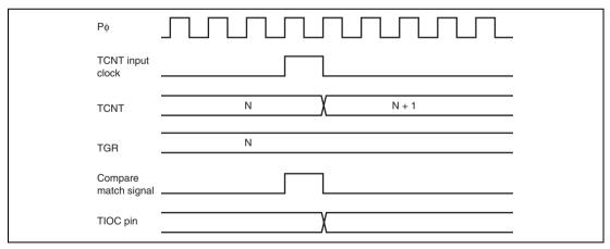
**Figure 10.97 Output Compare Output Timing (Normal Mode/PWM Mode)**
