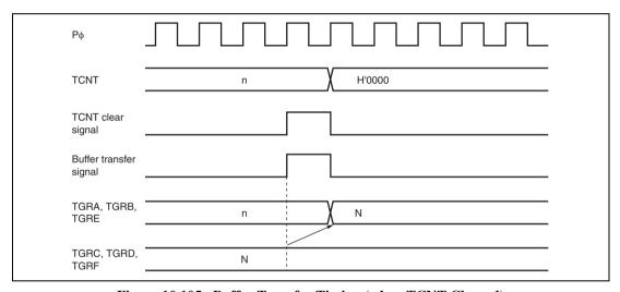
Figure 10.105 Buffer Transfer Timing (when TCNT Cleared)
