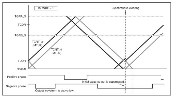
Figure 10.61 Example of Synchronous Clearing in Interval Tb at Trough (Timing (11) in Figure 10.56; Bit WRE of TWCR is 1)
