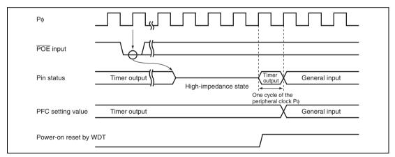
Figure 12.5 Pin Status When Power-on Reset is Issued from Watchdog Timer
