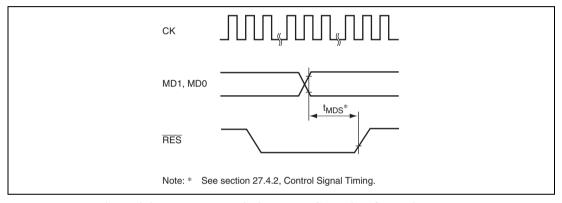
Figure 3.3 Reset Input Timing when Changing Operating Mode
