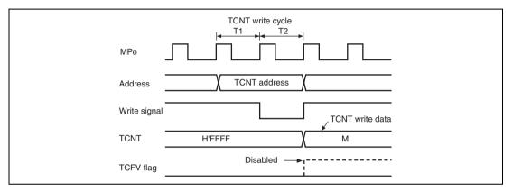
Figure 10.134 Contention between TCNT Write and Overflow
