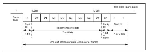
Figure 15.2 Example of Data Format in Asynchronous Communication (8-Bit Data with Parity and Two Stop Bits)
