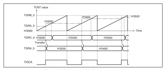
Figure 10.17 Example of Buffer Operation (1)
