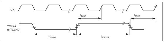
Figure 27.43 MTU2, MTU2S Clock Input Timing
