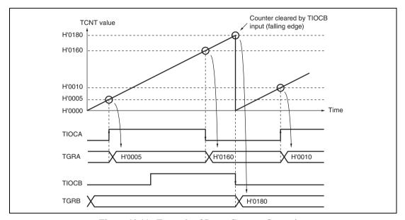
Figure 10.11 Example of Input Capture Operation
