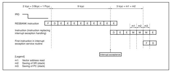
Figure 6.7 Example of Pipeline Operation when Interrupt is Accepted during RESBANK Instruction Execution (Register Banking without Register Bank Overflow)
