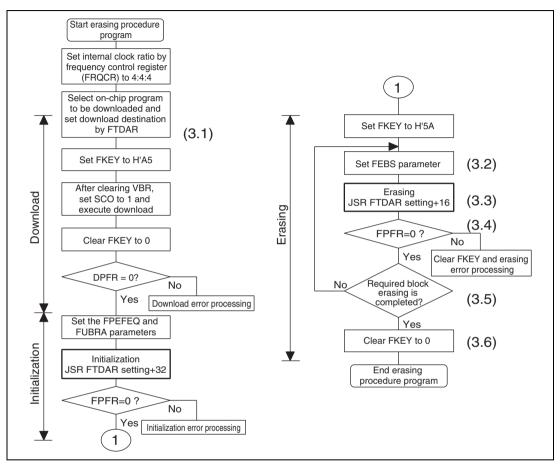
Figure 21.12 Erasing Procedure
