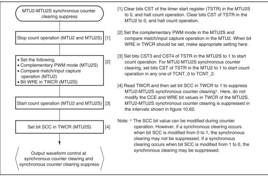
Figure 10.63 Example of Procedure for Suppressing MTU2–MTU2S Synchronous Counter Clearing
