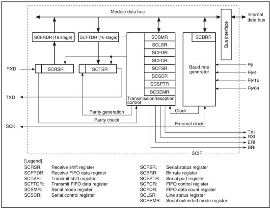
Figure 15.1 Block Diagram of SCIF
