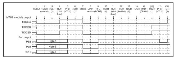
Figure 10.139 Error Occurrence in Normal Mode, Recovery in Complementary PWM Mode
