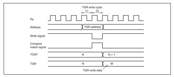
Figure 10.121 Contention between TGR Write and Compare Match
