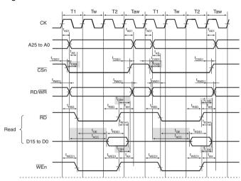
Figure 27.17 Bus Cycle 1104 of SRAM with Byte Selection (SW = 1 Cycle, HW = 1 Cycle, One Asynchronous External Wait Cycle, BAS = 0 (Write Cycle UB/LB Control))
