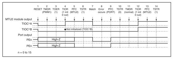
Figure 10.141 Error Occurrence in PWM Mode 1, Recovery in Normal Mode
