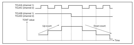
Figure 10.31 Example of Phase Counting Mode 2 Operation
