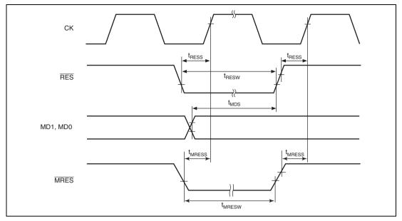
Figure 27.8 Reset Input Timing
