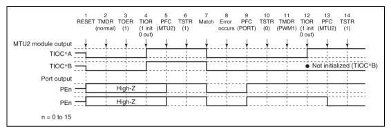
Figure 10.136 Error Occurrence in Normal Mode, Recovery in PWM Mode 1
