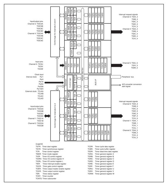
Figure 10.1 Block Diagram of MTU2
