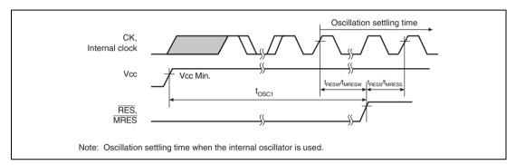
Figure 27.5 Power-On Oscillation Settling Time
