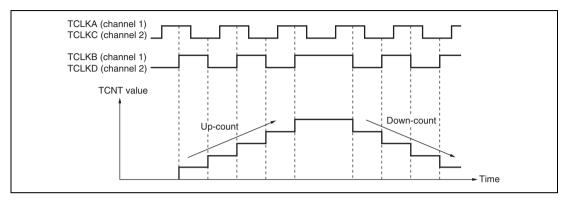
Figure 10.33 Example of Phase Counting Mode 4 Operation
