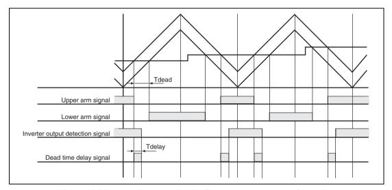
Figure 10.89 Delay in Dead Time in Complementary PWM Operation
