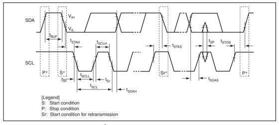
Figure 27.48 I<sup>2</sup>C Bus Interface 3 Input/Output Timing
