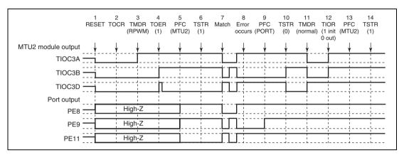
Figure 10.160 Error Occurrence in Reset-Synchronized PWM Mode, Recovery in Normal Mode
