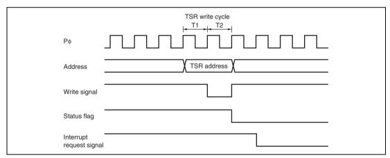
Figure 10.115 Timing for Status Flag Clearing by CPU (Channels 0 to 4)
