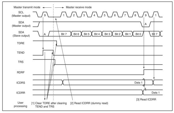
Figure 16.7 Master Receive Mode Operation Timing (1)
