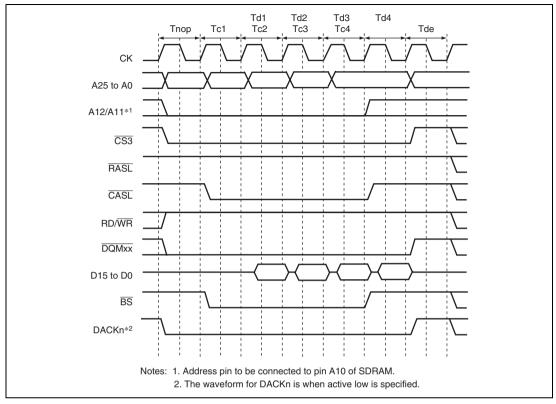
Figure 8.20 Burst Read Timing (Bank Active, Same Row Addresses in the Same Bank, CAS Latency 1)
