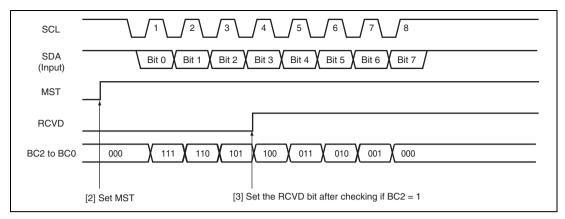
Figure 16.16 Operation Timing For Receiving One Byte (MST = 1)
