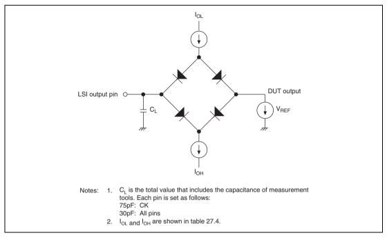
Figure 27.53 Output Load Circuit
