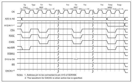
Figure 8.29 SDRAM Mode Write Timing (Based on JEDEC)
