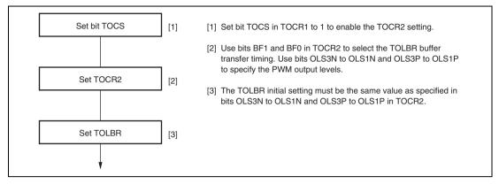
Figure 10.3 PWM Output Level Setting Procedure in Buffer Operation
