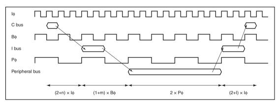
Figure 8.42 Internal Peripheral I/O Register Timing when Iφ:Βφ:Ρφ = 4:2:1
