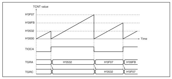
Figure 10.18 Example of Buffer Operation (2)
