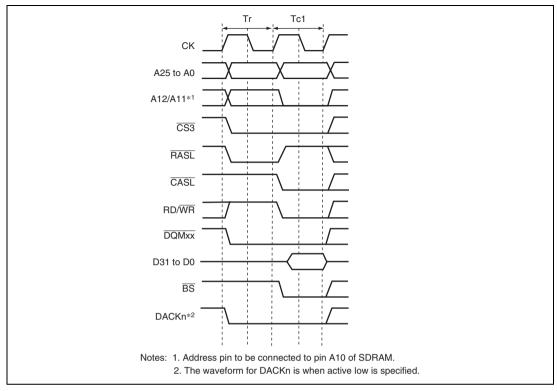
Figure 8.22 Single Write Timing (Bank Active, Different Bank)
