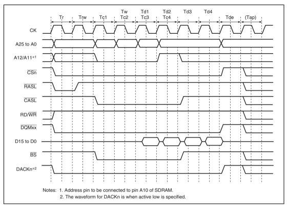
Figure 8.15 Burst Read Wait Specification Timing (CAS Latency 2, WTRCD[1:0] = 1 Cycle, Auto-Precharge)
