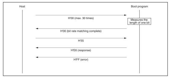
Figure 21.20 Sequence of Bit-Rate Matching
