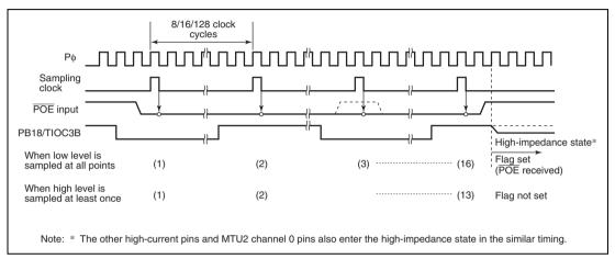
Figure 12.3 Low-Level Detection Operation
