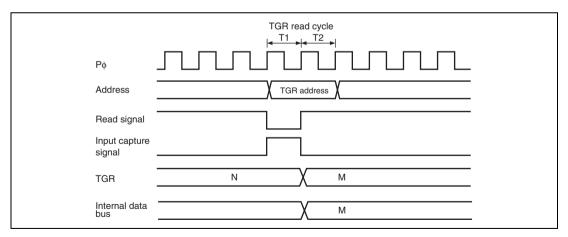
Figure 10.125 Contention between TGR Read and Input Capture (Channel 5)
