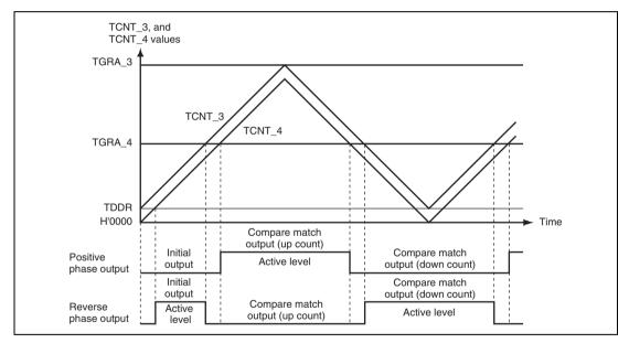
Figure 10.2 Complementary PWM Mode Output Level Example
