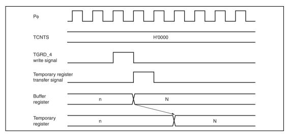
Figure 10.106 Transfer Timing from Buffer Register to Temporary Register (TCNTS Stop)
