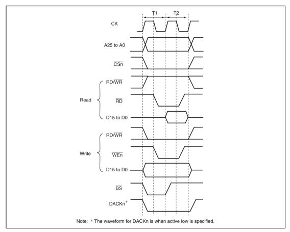
Figure 8.2 Normal Space Basic Access Timing (Access Wait 0)
