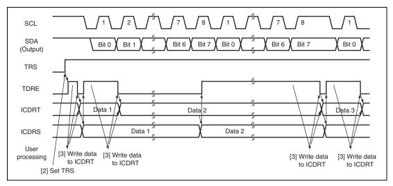
Figure 16.14 Transmit Mode Operation Timing
