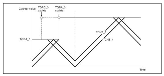
Figure 10.42 Example of PWM Cycle Updating
