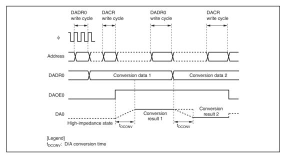
Figure 18.2 Example of D/A Converter Operation
