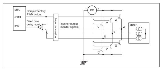
Figure 10.91 Example of Motor Control Circuit Configuration
