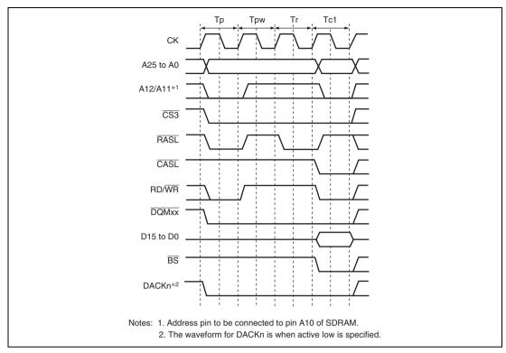
Figure 8.24 Single Write Timing (Bank Active, Different Row Addresses in the Same Bank)
