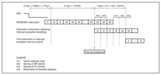
Figure 6.9 Example of Pipeline Operation when Interrupt is Accepted during RESBANK Instruction Execution (Register Banking with Register Bank Overflow)
