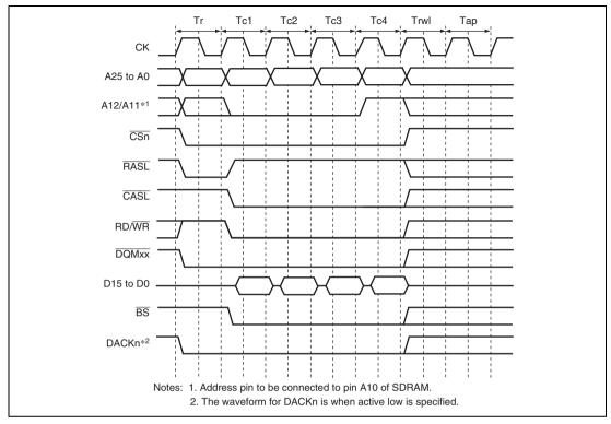
Figure 8.17 Basic Timing for Burst Write (Auto-Precharge)
