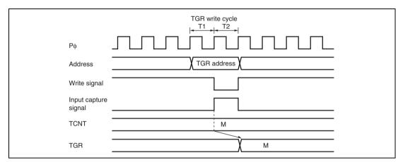
Figure 10.126 Contention between TGR Write and Input Capture (Channels 0 to 4)
