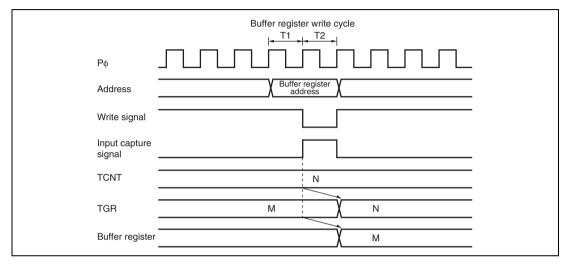
Figure 10.128 Contention between Buffer Register Write and Input Capture
