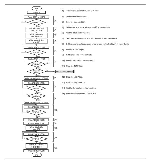
Figure 16.18 Sample Flowchart for Master Transmit Mode
