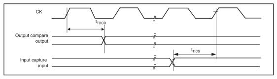
Figure 27.42 MTU2, MTU2S Input/Output Timing
