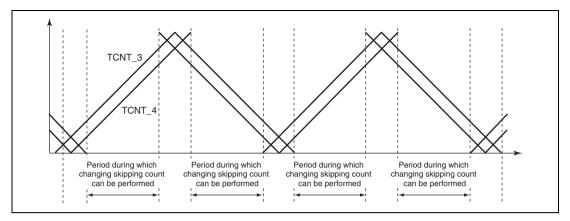
Figure 10.74 Periods during which Interrupt Skipping Count can be Changed
