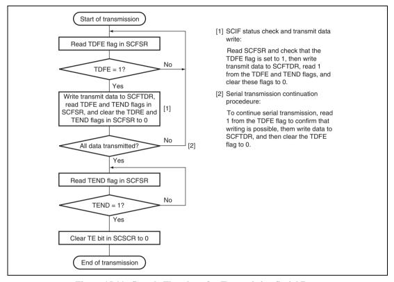
Figure 15.11 Sample Flowchart for Transmitting Serial Data
