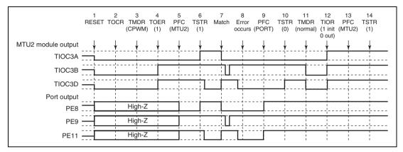
Figure 10.155 Error Occurrence in Complementary PWM Mode, **Recovery in Normal Mode**
