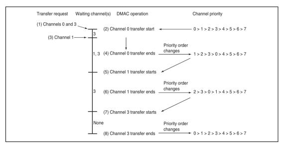
Figure 9.4 Changes in Channel Priority in Round-Robin Mode
