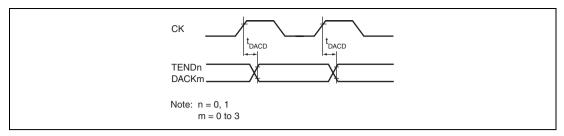
Figure 27.41 DACK, TEND Output Timing
