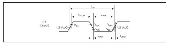
Figure 27.4 CK Clock Output Timing
