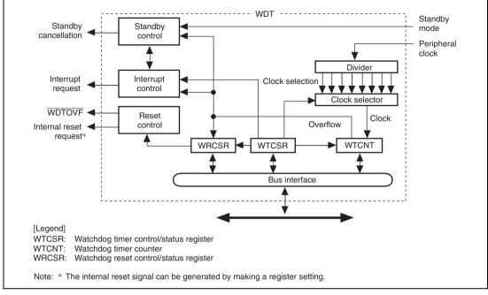
Figure 14.1 Block Diagram of WDT
