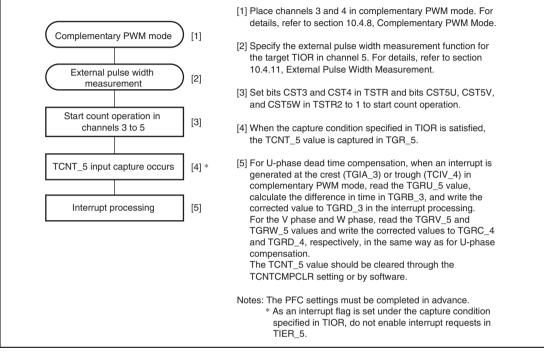
Figure 10.90 Example of Dead Time Compensation Setting Procedure
