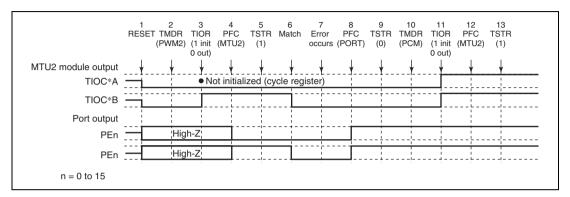
Figure 10.150 Error Occurrence in PWM Mode 2, Recovery in Phase Counting Mode
