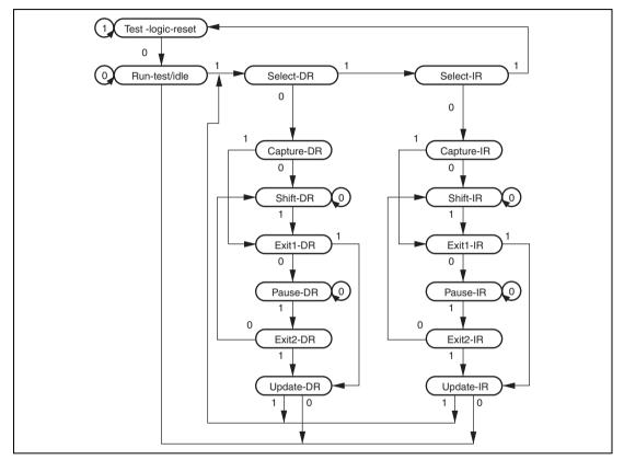
Figure 24.2 TAP Controller State Transitions
