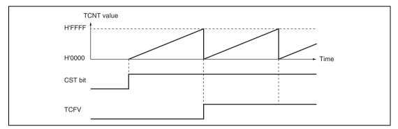
Figure 10.5 Free-Running Counter Operation
