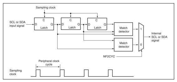
Figure 16.17 Block Diagram of Noise Filter
