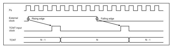
Figure 10.96 Count Timing in External Clock Operation (Phase Counting Mode)
