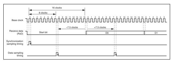
Figure 15.17 Receive Data Sampling Timing in Asynchronous Mode
