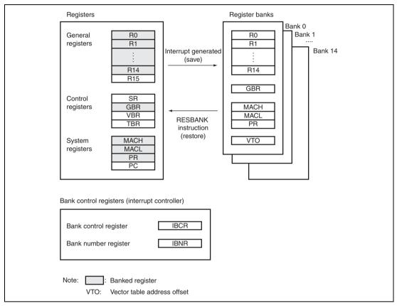
Figure 6.10 Overview of Register Bank Configuration
