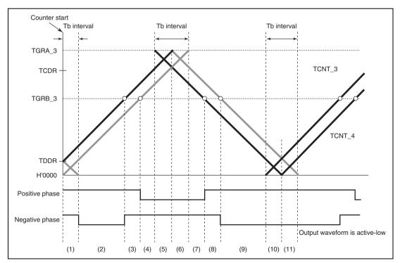
Figure 10.56 Timing for Synchronous Counter Clearing
