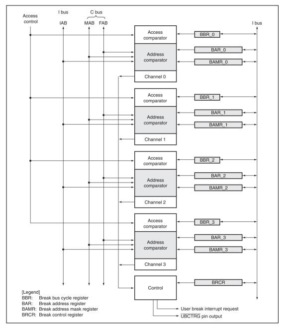
Figure 7.1 Block Diagram of UBC
