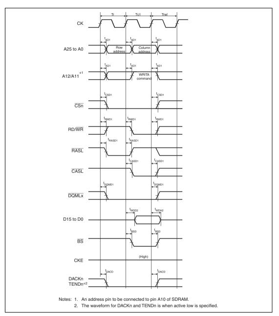
Figure 27.24 Synchronous DRAM Single Write Bus Cycle (Auto Precharge, TRWL = 1 Cycle)
