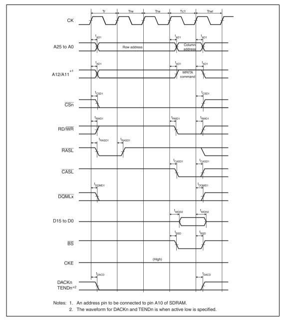
Figure 27.25 Synchronous DRAM Single Write Bus Cycle (Auto Precharge, WTRCD = 2 Cycles, TRWL = 1 Cycle)
