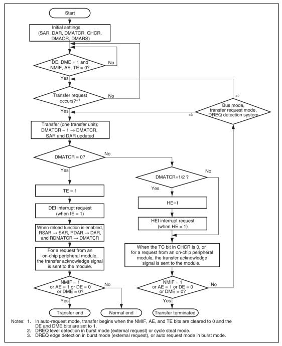
Figure 9.2 DMA Transfer Flowchart
