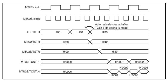
Figure 10.84 (2) Example of Synchronous Counter Start Operation (MTU2-to-MTU2S Clock Frequency Ratio = 1:2)
