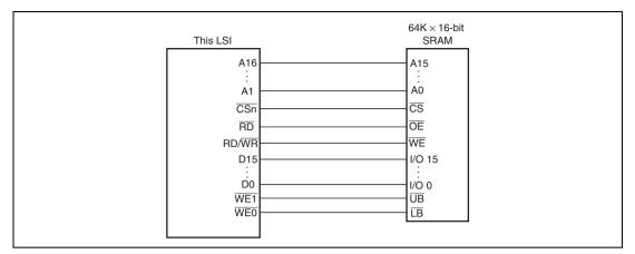
Figure 8.36 Example of Connection with 16-Bit Data-Width SRAM with Byte Selection
