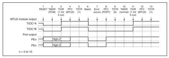
Figure 10.151 Error Occurrence in Phase Counting Mode, Recovery in Normal Mode
