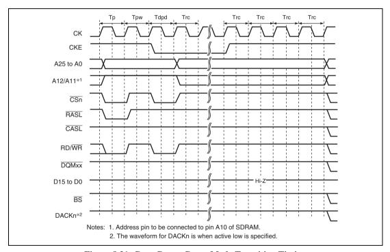
Figure 8.31 Deep Power-Down Mode Transition Timing
