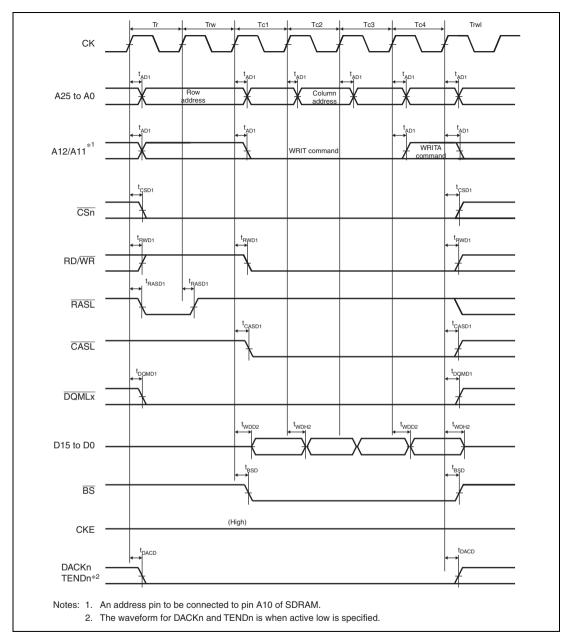
Figure 27.27 Synchronous DRAM Burst Write Bus Cycle (Four Write Cycles)
