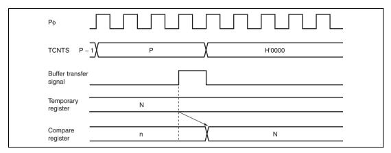
Figure 10.108 Transfer Timing from Temporary Register to Compare Register
