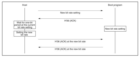
Figure 21.22 Sequence of New Bit Rate Selection
