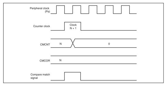
Figure 13.4 Timing of CMF Setting
