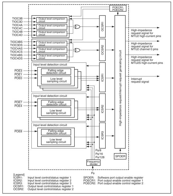
Figure 12.1 Block Diagram of POE2
