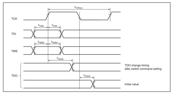
Figure 27.52 H-UDI Data Transfer Timing
