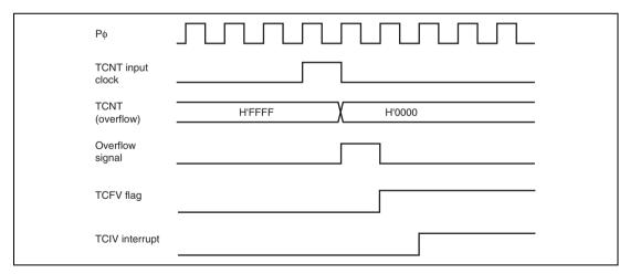
Figure 10.113 TCIV Interrupt Setting Timing
