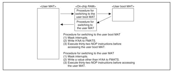
Figure 21.17 Switching between User MAT and User Boot MAT
