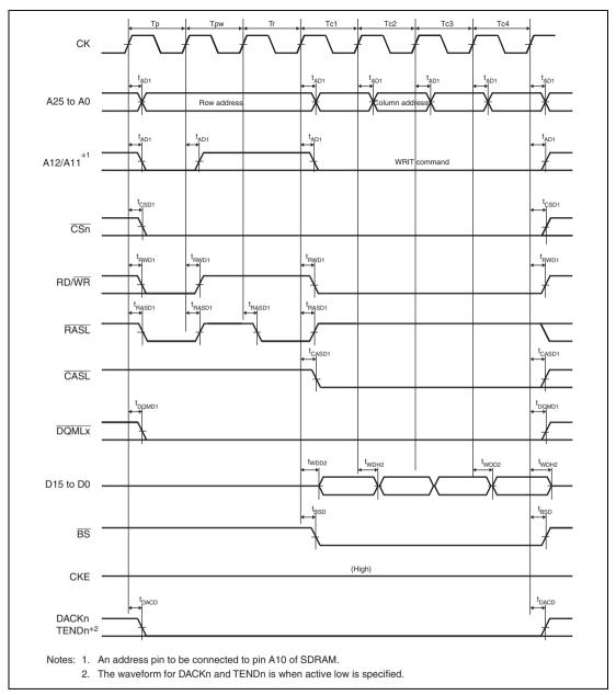
Figure 27.33 Synchronous DRAM Burst Write Bus Cycle (Four Write Cycles)
