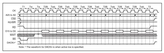
Figure 8.37 Burst ROM Access Timing (Clock Synchronous)
