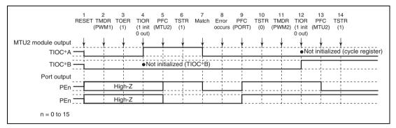
Figure 10.143 Error Occurrence in PWM Mode 1, Recovery in PWM Mode 2
