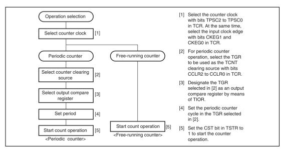
Figure 10.4 Example of Counter Operation Setting Procedure
