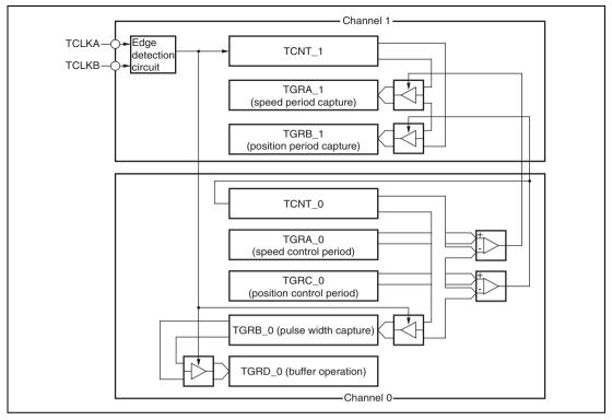
Figure 10.34 Phase Counting Mode Application Example
