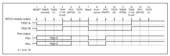
Figure 10.138 Error Occurrence in Normal Mode, Recovery in Phase Counting Mode
