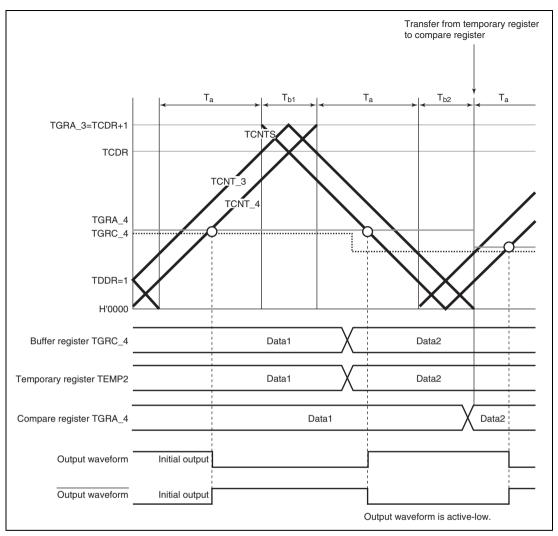
Figure 10.41 Example of Operation without Dead Time
