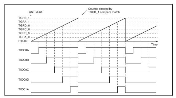
Figure 10.27 Example of PWM Mode Operation (2)
