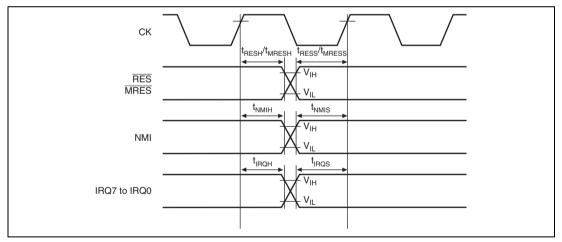
Figure 27.9 Interrupt Signal Input Timing
