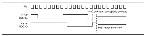
Figure 12.4 Output-Level Compare Operation
