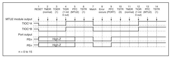
Figure 10.135 Error Occurrence in Normal Mode, Recovery in Normal Mode
