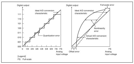
Figure 17.7 Definitions of A/D Conversion Accuracy
