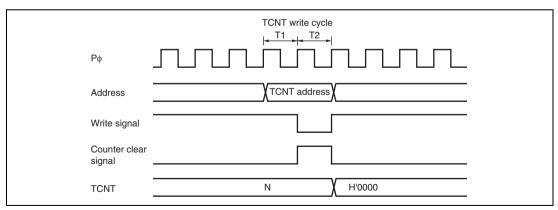
Figure 10.119 Contention between TCNT Write and Clear Operations
