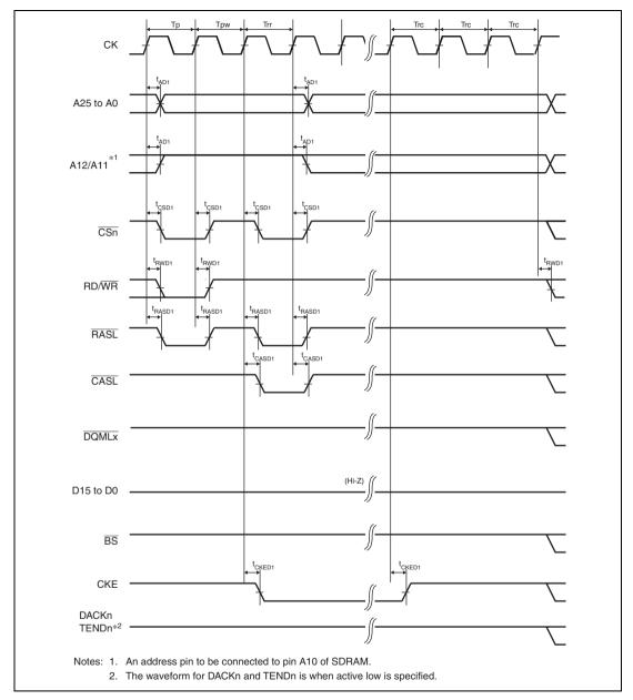
Figure 27.35 Synchronous DRAM Self-Refreshing Timing (WTRP = 1 Cycle)
