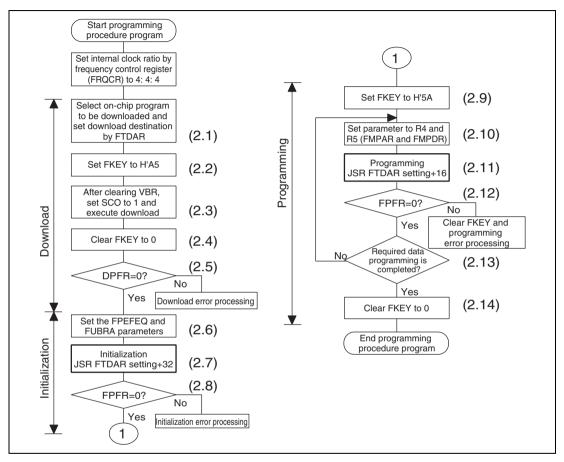
Figure 21.11 Programming Procedure
