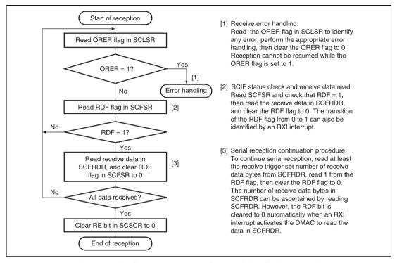
Figure 15.13 Sample Flowchart for Receiving Serial Data (1)
