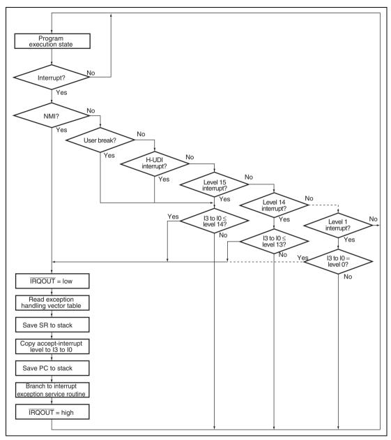
Figure 6.2 Interrupt Operation Flow
