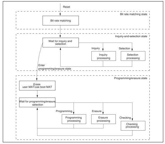
Figure 21.19 Flow of Processing by the Boot Program
