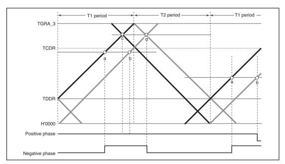
$Figure\ 10.47\quad Example\ of\ Complementary\ PWM\ Mode\ Waveform\ Output\ (2)$
