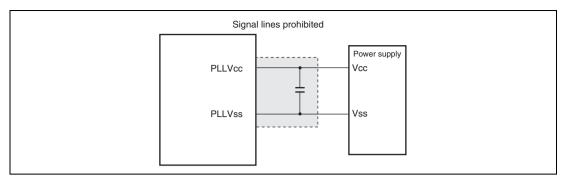
Figure 4.3 Note on Using a PLL Oscillation Circuit
