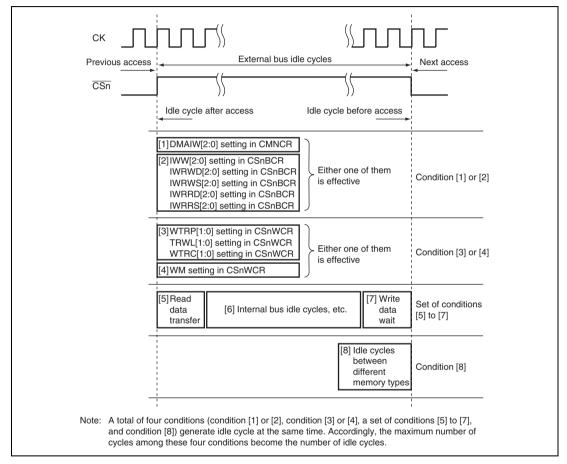
Figure 8.38 Idle Cycle Conditions
