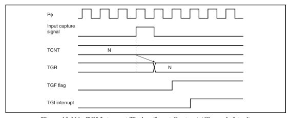
Figure 10.111 TGI Interrupt Timing (Input Capture) (Channels  $0\ to\ 4)$
