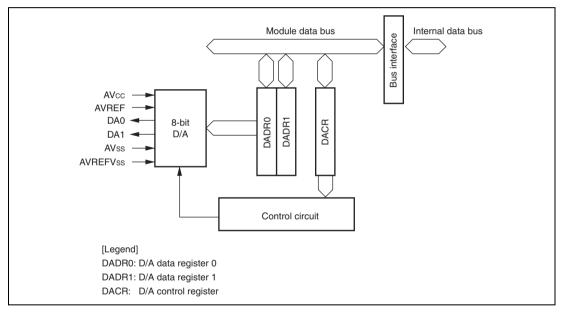
Figure 18.1 Block Diagram of D/A Converter
