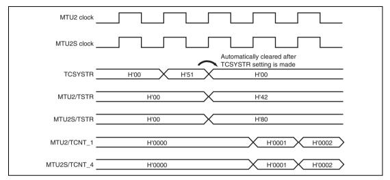
Figure 10.84 (1) Example of Synchronous Counter Start Operation (MTU2-to-MTU2S Clock Frequency Ratio = 1:1)
