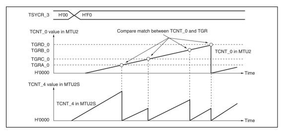
Figure 10.86 (2) Example of MTU2S Counter Clearing Caused by MTU2 Flag Setting Source (2)
