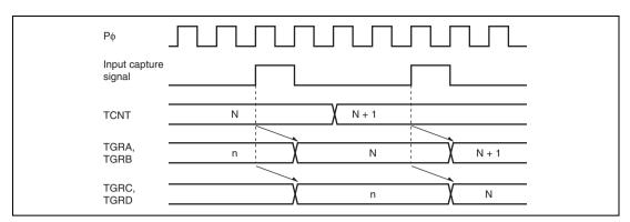
Figure 10.104 Buffer Operation Timing (Input Capture)
