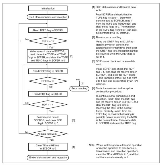
Figure 15.16 Sample Flowchart for Transmitting/Receiving Serial Data
