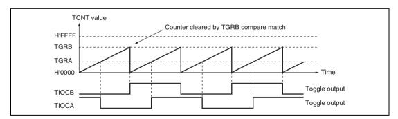
Figure 10.9 Example of Toggle Output Operation
