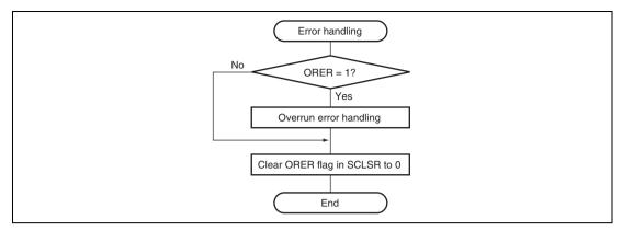
Figure 15.14 Sample Flowchart for Receiving Serial Data (2)
