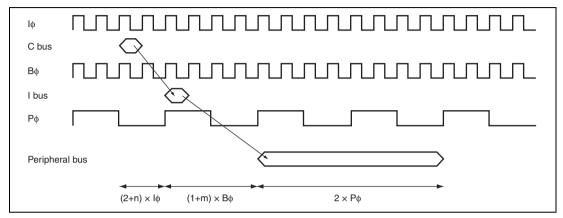
Figure 8.41 Internal Peripheral I/O Register Timing when  $I\phi:B\phi:P\phi=4:4:1$
