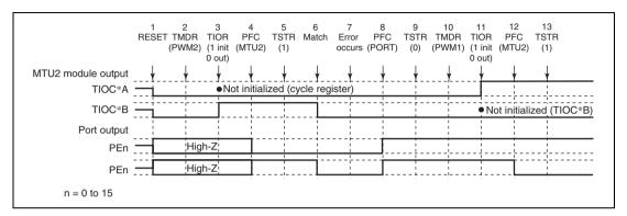
Figure 10.148 Error Occurrence in PWM Mode 2, Recovery in PWM Mode 1
