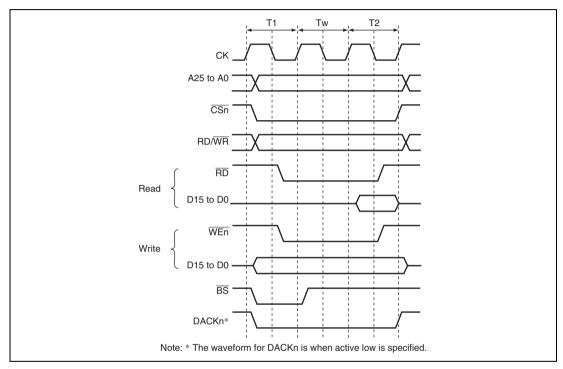
Figure 8.7 Wait Timing for Normal Space Access (Software Wait Only)
