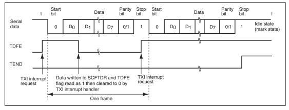
Figure 15.5 Example of Transmit Operation (8-Bit Data, Parity, 1 Stop Bit)
