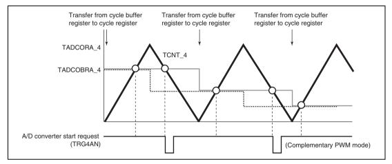
Figure 10.80 Basic Example of A/D Converter Start Request Signal (TRG4AN) Operation
