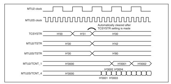
Figure 10.84 (4) Example of Synchronous Counter Start Operation (MTU2-to-MTU2S Clock Frequency Ratio = 1:4)
