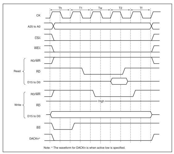
Figure 8.35 Wait Timing for SRAM with Byte Selection (BAS = 1) (SW[1:0] = 01, WR[3:0] = 0001, HW[1:0] = 01)
