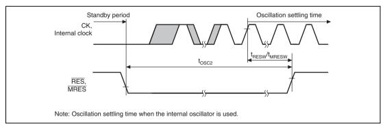
Figure 27.6 Oscillation Settling Time on Return from Standby (Return by Reset)
