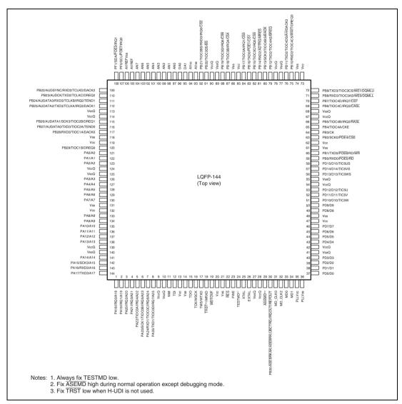
Figure 1.2 Pin Arrangement
