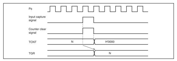
Figure 10.102 Counter Clear Timing (Input Capture) (Channels 0 to 5)
