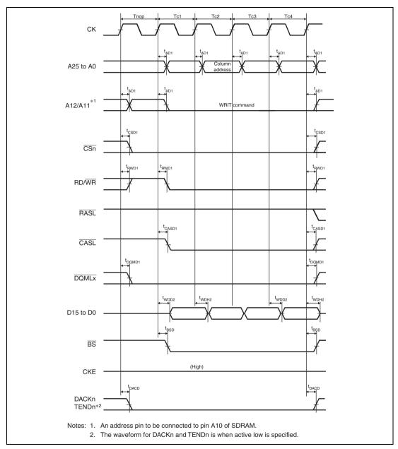
Figure 27.32 Synchronous DRAM Burst Write Bus Cycle (Four Write Cycles)
