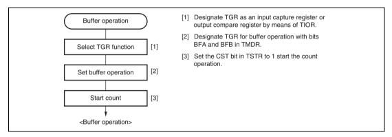
Figure 10.16 Example of Buffer Operation Setting Procedure
