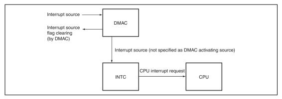
Figure 6.13 Interrupt Control Block Diagram
