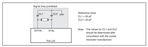
Figure 4.2 Note on Using a Crystal Resonator
