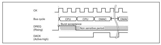
Figure 9.15 Example of DREQ Input Detection in Burst Mode Edge Detection
