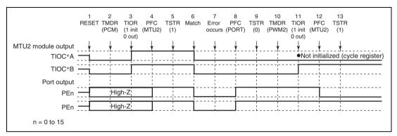
Figure 10.153 Error Occurrence in Phase Counting Mode, Recovery in PWM Mode 2
