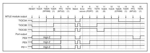
Figure 10.162 Error Occurrence in Reset-Synchronized PWM Mode, Recovery in Complementary PWM Mode
