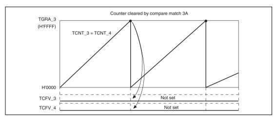
Figure 10.132 Reset Synchronous PWM Mode Overflow Flag
