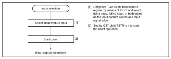
Figure 10.10 Example of Input Capture Operation Setting Procedure
