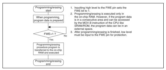
Figure 21.9 Programming/Erasing Overview Flow
