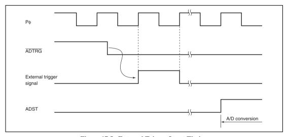
Figure 17.5 External Trigger Input Timing
