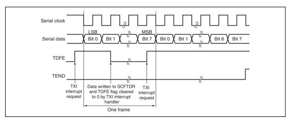
Figure 15.12 Example of SCIF Transmit Operation
