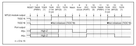
Figure 10.142 Error Occurrence in PWM Mode 1, Recovery in PWM Mode 1
