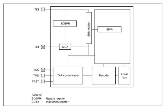
Figure 24.1 Block Diagram of H-UDI
