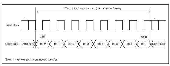
Figure 15.9 Data Format in Clocked Synchronous Communication
