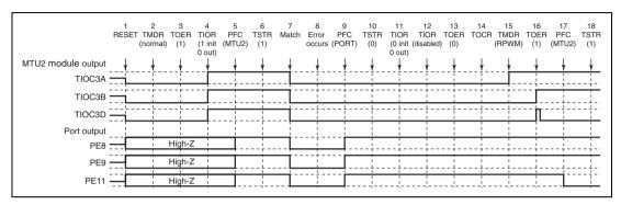
Figure 10.140 Error Occurrence in Normal Mode, Recovery in Reset-Synchronized PWM Mode
