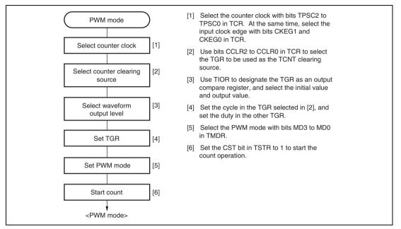
Figure 10.25 Example of PWM Mode Setting Procedure
