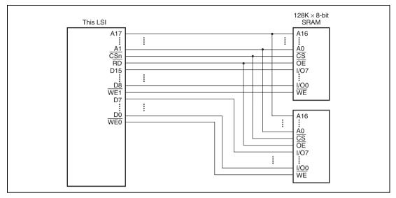
Figure 8.5 Example of 16-Bit Data-Width SRAM Connection
