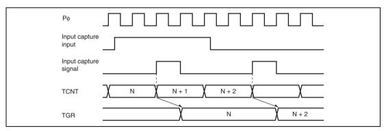
Figure 10.99 Input Capture Input Signal Timing
