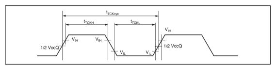
Figure 27.51 TCK Input Timing
