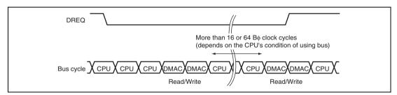
Figure 9.10 Example of DMA Transfer in Cycle-Steal Intermittent Mode (Dual Address, DREQ Low Level Detection)
