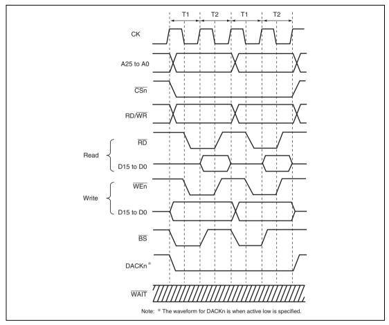
Figure 8.4 Continuous Access for Normal Space 2
