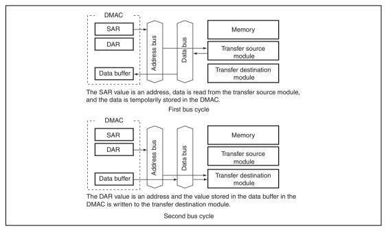
Figure 9.5 Data Flow of Dual Address Mode
