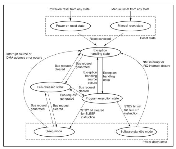
Figure 2.6 Transitions between Processing States
