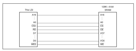
Figure 8.6 Example of 8-Bit Data-Width SRAM Connection
