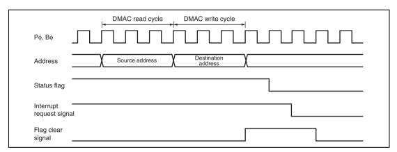
Figure 10.117 Timing for Status Flag Clearing by DTC Activation (Channels 0 to 4)
