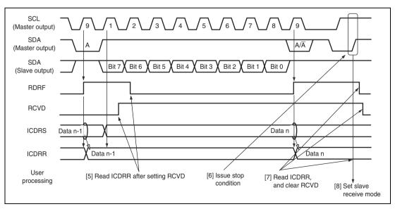
Figure 16.8 Master Receive Mode Operation Timing (2)
