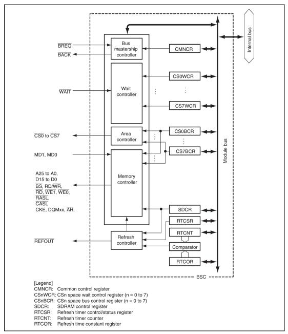
Figure 8.1 Block Diagram of BSC
