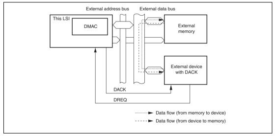
Figure 9.7 Data Flow in Single Address Mode
