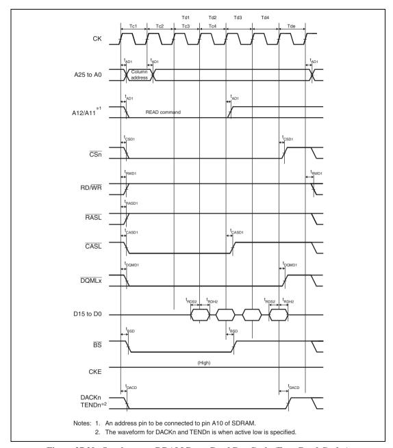
Figure 27.29 Synchronous DRAM Burst Read Bus Cycle (Four Read Cycles)
