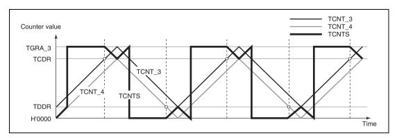
Figure 10.39 Complementary PWM Mode Counter Operation
