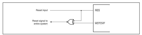
Figure 14.6 Example of System Reset Circuit Using WDTOVF Signal
