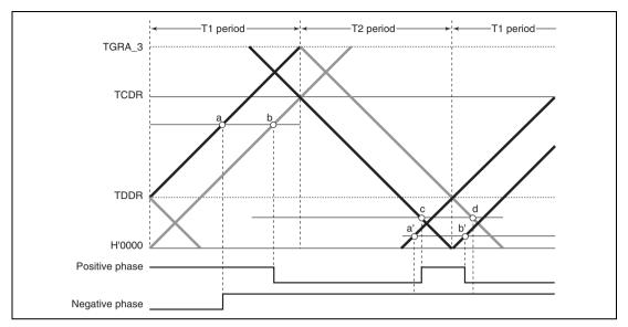
Figure 10.48 Example of Complementary PWM Mode Waveform Output (3)
