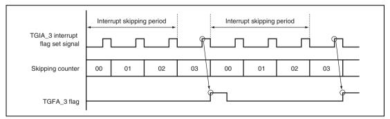
Figure 10.75 Example of Interrupt Skipping Operation
