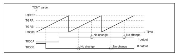
Figure 10.8 Example of 0 Output/1 Output Operation
