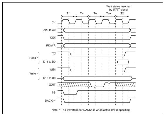
Figure 8.8 Wait Cycle Timing for Normal Space Access (Wait Cycle Insertion Using WAIT Signal)
