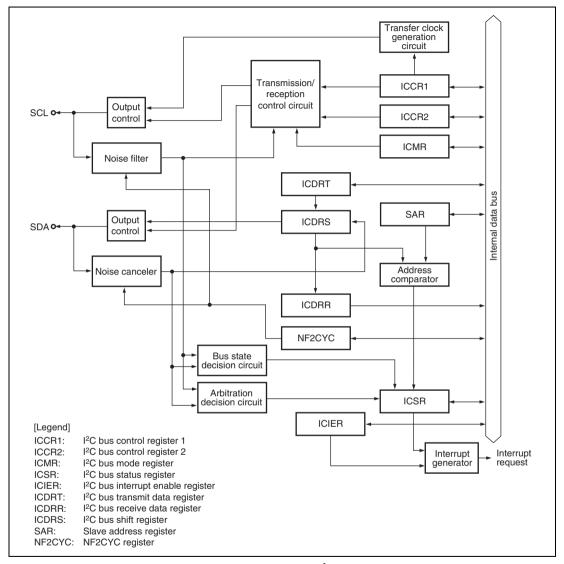
Figure 16.1 Block Diagram of I<sup>2</sup>C Bus Interface 3
