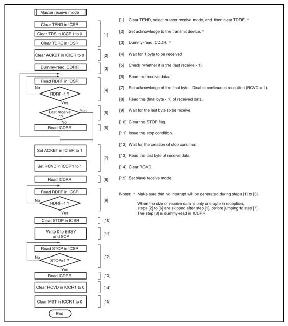
Figure 16.19 Sample Flowchart for Master Receive Mode
