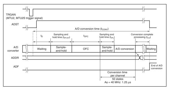
Figure 17.4 A/D Conversion Timing (Single-Cycle Scan Mode)
