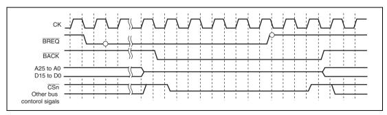
Figure 8.40 Bus Arbitration Timing (Clock Mode 7 or CMNCR.HIZCNT = 1)
