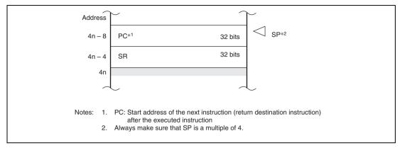
Figure 6.3 Stack after Interrupt Exception Handling
