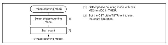
Figure 10.29 Example of Phase Counting Mode Setting Procedure
