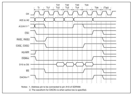
Figure 8.14 Burst Read Basic Timing (CAS Latency 1, Auto-Precharge)
