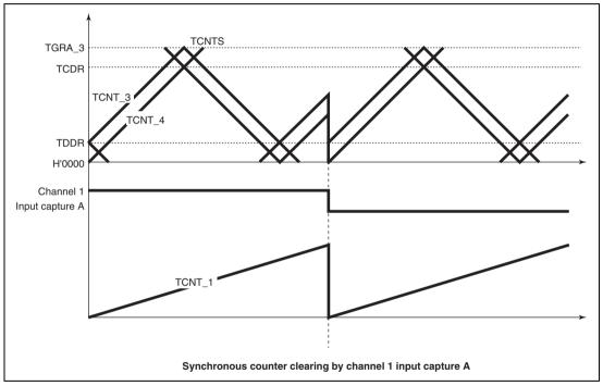
Figure 10.55 Counter Clearing Synchronized with Another Channel
