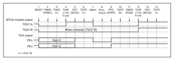
Figure 10.144 Error Occurrence in PWM Mode 1, Recovery in Phase Counting Mode
