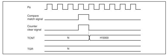
Figure 10.100 Counter Clear Timing (Compare Match) (Channels 0 to 4)
