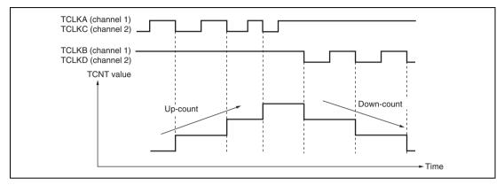
Figure 10.32 Example of Phase Counting Mode 3 Operation
