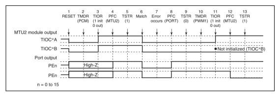
Figure 10.152 Error Occurrence in Phase Counting Mode, Recovery in PWM Mode 1
