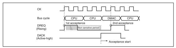
Figure 9.13 Example of DREQ Input Detection in Cycle Steal Mode Edge Detection
