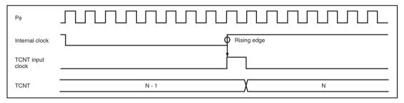
Figure 10.94 Count Timing in Internal Clock Operation (Channel 5)
