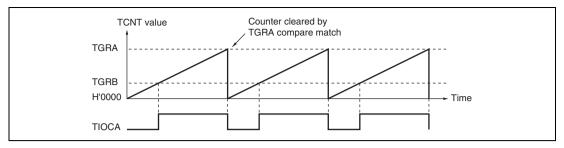
Figure 10.26 Example of PWM Mode Operation (1)
