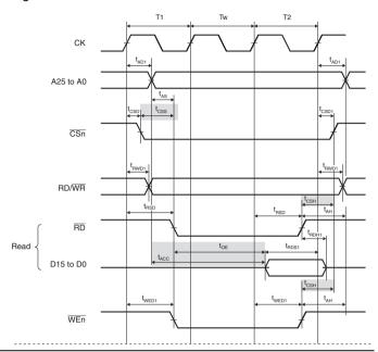
Figure 27.14 Basic Bus 1101 Timing for Normal Space (One External Wait Cycle)
