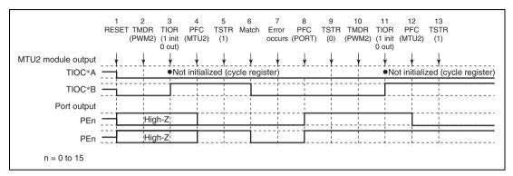
Figure 10.149 Error Occurrence in PWM Mode 2, Recovery in PWM Mode 2
