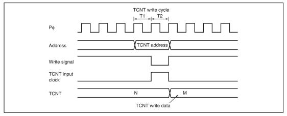
Figure 10.120 Contention between TCNT Write and Increment Operations
