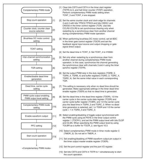
Figure 10.38 Example of Complementary PWM Mode Setting Procedure
