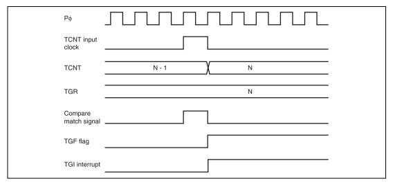
Figure 10.110 TGI Interrupt Timing (Compare Match) (Channel 5)
