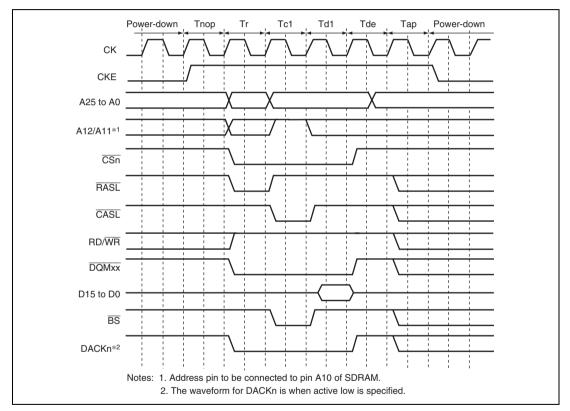
Figure 8.28 Power-Down Mode Access Timing
