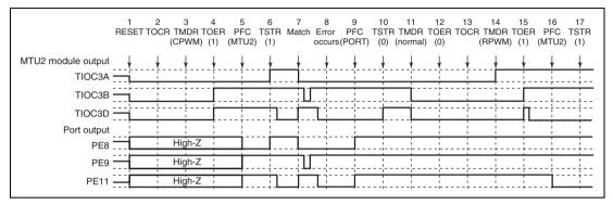
Figure 10.159 Error Occurrence in Complementary PWM Mode, Recovery in Reset-Synchronized PWM Mode
