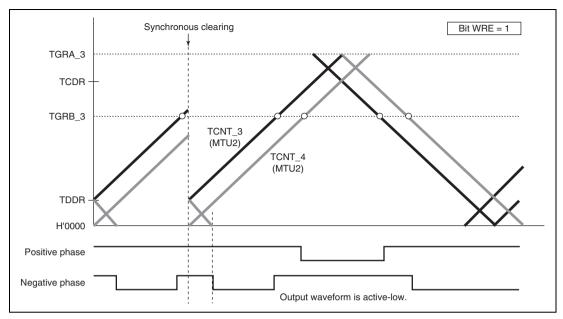
Figure 10.58 Example of Synchronous Clearing in Dead Time during Up-Counting (Timing (3) in Figure 10.56; Bit WRE of TWCR in MTU2 is 1)
