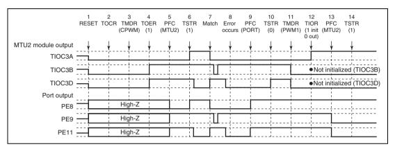
Figure 10.156 Error Occurrence in Complementary PWM Mode, Recovery in PWM Mode 1
