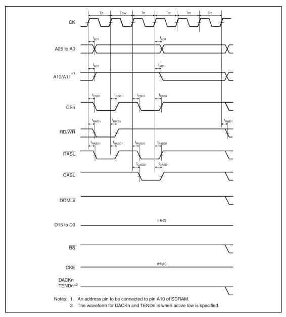
Figure 27.34 Synchronous DRAM Auto-Refreshing Timing (WTRP = 1 Cycle, WTRC = 3 Cycles)
