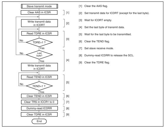
Figure 16.20 Sample Flowchart for Slave Transmit Mode
