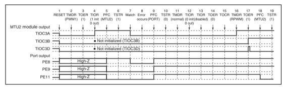
Figure 10.146 Error Occurrence in PWM Mode 1, Recovery in Reset-Synchronized PWM Mode
