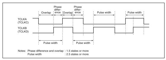
Figure 10.118 Phase Difference, Overlap, and Pulse Width in Phase Counting Mode
