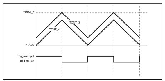
Figure 10.54 Example of Toggle Output Waveform Synchronized with PWM Output
