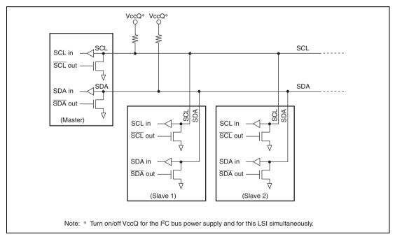
Figure 16.2 External Circuit Connections of I/O Pins
