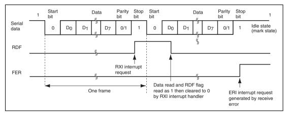
Figure 15.8 Example of SCIF Receive Operation (8-Bit Data, Parity, 1 Stop Bit)
