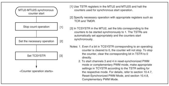
Figure 10.83 Example of Synchronous Counter Start Setting Procedure
