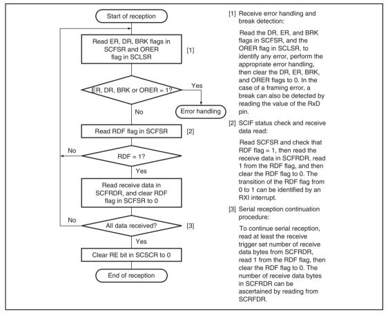
Figure 15.6 Sample Flowchart for Receiving Serial Data
