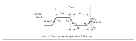
Figure 27.3 EXTAL Clock Input Timing
